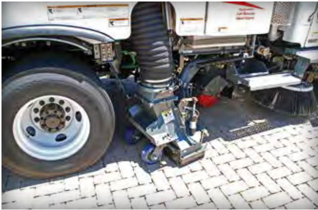
Figure 22. A true vacuum machine cleaning neglected PICP.
