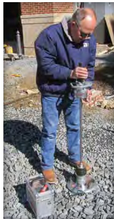
Figure 22. Testing base stiffness using light-weight deflectometer.
