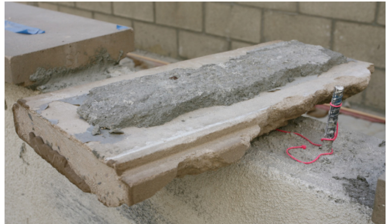
THE ADDED FLEXURAL BOND WAS STRONGER THAN THE PRECAST CONCRETE ITSELF. CONVENTIONAL POLYMER CEMENT MORTARS HAD FAILED IN BONDING THESE CANTILEVERED WALL CAPS.
