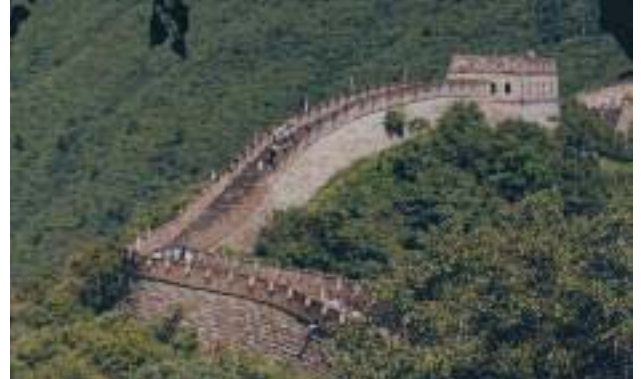
The Great Wall of China, dating back some 2,200 years, was built as a double sided retaining wall. The soil between the two walls was a mixture of clay and gravel reinforced with Tamarisk branches. Allan Block retaining walls employ "old technology with new materials."
