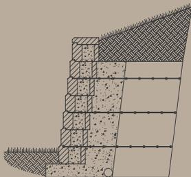
**Chart Example:** A 5 ft. (1.5 m) tall wall in sandy soil with a level surface above can be built with AB Stones of the AB Collection and would typically not require reinforcement, but will require review by a local professional engineer.
