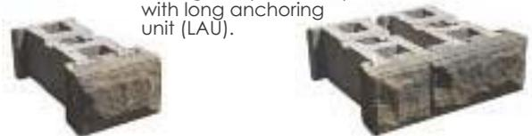
The **short anchoring unit (SAU)** is used for lower height gravity walls and reinforced walls. Walls taller than those listed in the Maximum Gravity Wall Heights Chart on page 10 will need geogrid reinforcement for additional stability. Refer to page 22 for general reinforcement requirements and instructions.
