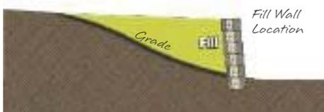
A "fill" site is where you will need extra soils to fill in behind the entire wall. You will need to plan ahead to have good backfill materials brought onto the site.
