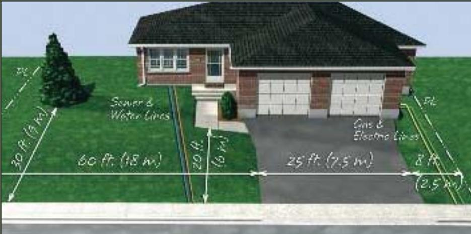
A detailed site plan drawn to scale will help foresee design and construction challenges and provide an accurate reference for estimating. This will become your working or approved plans for the project.
