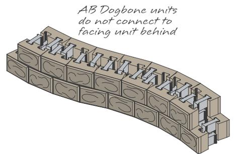
Parapet graphics are to show facing unit and AB Dogbone placements. All parapet installations need to include wall rock in cores.
