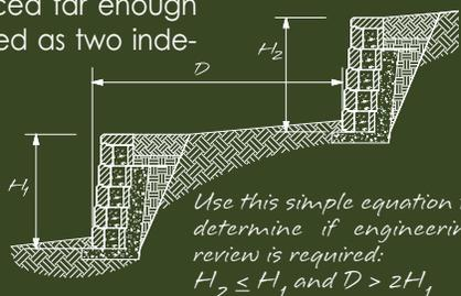
As the upper wall moves closer to the lower wall, it adds pressure (surcharge) to the lower wall.
