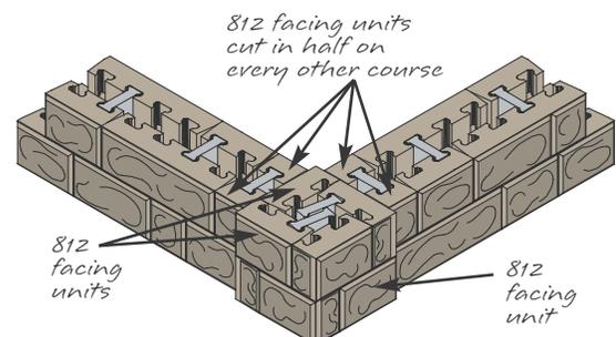
Parapet graphics are to show facing unit and AB Dogbone placements. All parapet installations need to include wall rock in cores.
