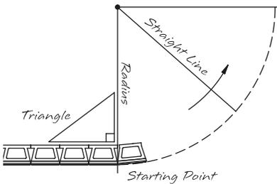
Attach a string line to the stake the length of the radius and rotate it around to mark the location of the base course. Install the blocks with the front of the blocks lining up with the mark.
