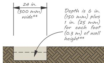
\*\* For walls under 4 ft. (1.2 m) dig the base trench 18 in. wide (460 mm) and 4 in. deep (100 mm) plus additional to account for the amount of buried block needed.
