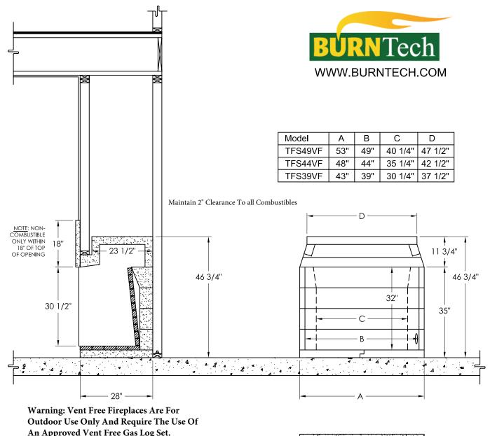
An Approved Vent Free Gas Log Set. Burning Wood In A Vent Free Unit Can Cause Serious Injury Or Death. Check With Your Local Building Officials For Approval Prior To Installation.
