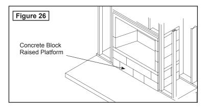
When determining raised hearth height, be sure to allow for the 3" thick firebox hearth and 1-1/2" thick firebrick floor, in addition to the height of base platform.
