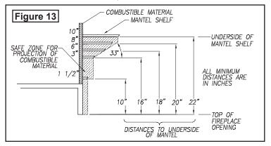
Parts of the combustible mantle assembly located above and projecting more than one and one-half inches (1-1/2")inches from the firebox opening shall be kept at least twelve inches (12") from the top of the opening.
