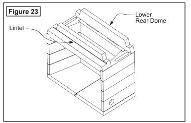
Although you are cautioned to use Burntech mortar 11) Place Lower Side Domes between Lintel and Lower Rear Dome to verify fit. The face with the rating plate faces the inside of the firebox as shown in Figure 24. Remove and prepare mating surfaces with mortar. Assemble Lower Dome Sides and check that all four top surfaces are level with each other. Shim if necessary.
