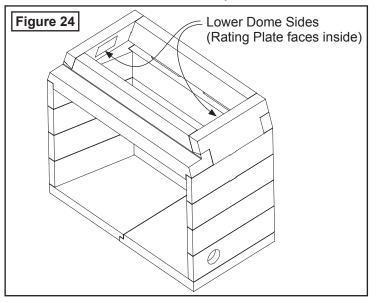
13) Now install the Smoke Dome Tops. Align outer edges with Lower Dome Sides. Check for flatness and squareness.
