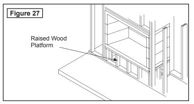
For a "flush hearth" (fireplace floor flush with the room's floor) the base plate can be omitted from the assembly and the firebox walls built directly on the concrete support slab. The fire brick floor of the firebox is then set directly to the concrete support slab. This makes the fireplace finished fire brick floor approximately one and one-half inches (1-1/2") above the top of the concrete support slab.
