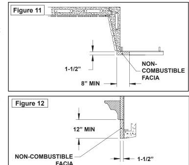
Clearance to combustible trim are those distances required to ensure that combustible mantle and facing material will not be exposed to excessive heat while the unit is operating.
