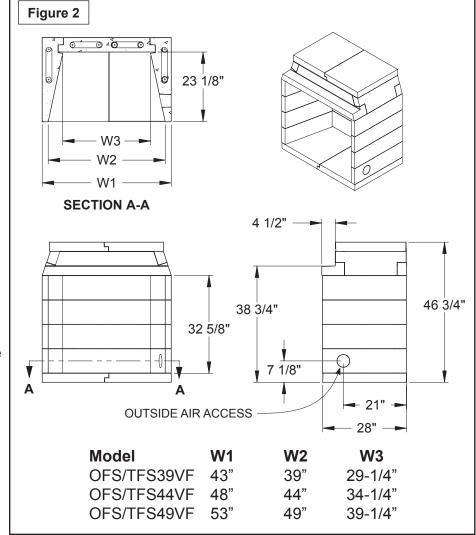
In addition to the basic enclosure, a standard 1-1/8" thick, high temperature refractory brick is required to line the interior of the firebox.
