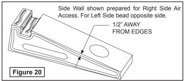
6) Keep the assembly of the next sections of the firebox side walls moving up, keeping components moist, mixing mortar as you need it and threading the mortar appropriately as you stack each section, one onto the next. Constantly check for squareness and levelness while building each course of block. As you complete each section, make certain that you adhere the mortar at each and every joint.
