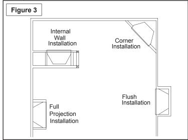
**A flush installation** is recommended where living space is limited or at a premium. Check local codes for any restrictions.
