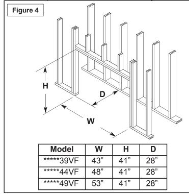
**Projected installations** can extend any distance into the room. A projection may be ideal for a new addition on an existing, finished wall.
