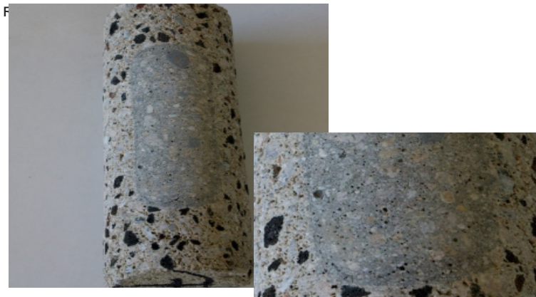
CORE SAMPLE OF GA213 SHOWING SUPERIOR BOND AND NON-SHRINK PROPERTIES
